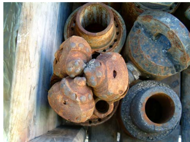
Collection of badly worn drilling bits
